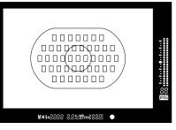
The 45-point AF unit is the same as the EOS-1D's. However, the AF-related circuitry and the AF algorithm incorporate a completely new design so that the AF performance surpasses that of the 1D. The EOS-1D had a single CPU for AF operations from focus detection to lens-driving control. The EOS-1D Mark II has two CPUs taking care of these functions.
