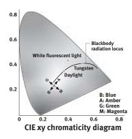
The Auto White Balance has been improved to obtain more precise color reproduction at low color temperatures such as tungsten and fluorescent light. The accuracy of the new algorithm has made it possible to eliminate the external AWB sensor and the need for hybrid AWB.
